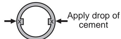
1. For Lock-Closed Only (prevents valve from being locked in the open position): cement lock ring on body stem tower with lugs aligned with valve and pipe line.
