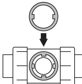
2. For Lock-Open Only (prevents valve from being locked in the closed position): cement lock ring on body stem tower with lugs perpendicular to valve and pipe line.
